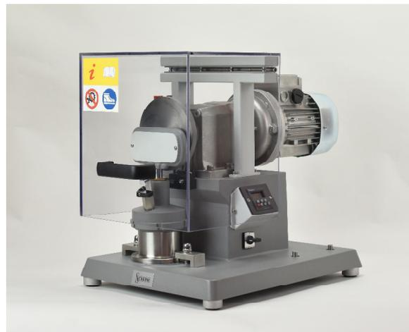
Single-unit grease working machine
