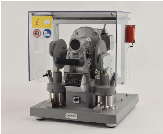
Dual-unit grease working machine
